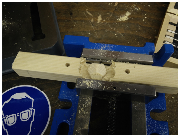
FIGURE 78 – Enlarged 6mm wide holes using the drill press
