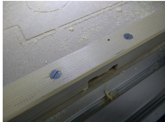
(b) Motherpiece correctly fastened to the buffer sheet
