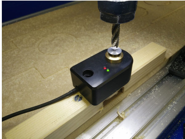
FIGURE 81 – Calibrating along the Z axis
