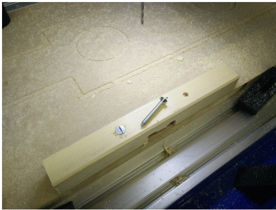
(a) Screws to be used to fasten the motherpiece on the buffer sheet
