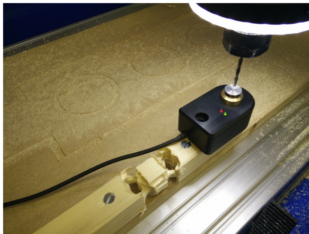
FIGURE 82 – Calibration along the Z axis for the 3.175mm tool
