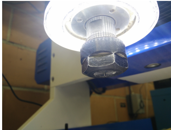
(c) Lock-nut correctly screwed onto the spindle
