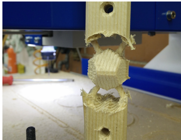
FIGURE 52 – Holding tabs used to fasten the finished part to it's mother piece
