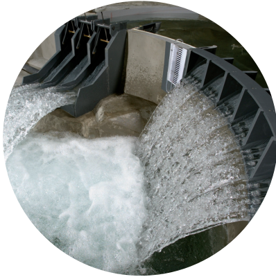
Scale model of the shahryar dam (Ostour, Iran) in lab LCH, EPFL
