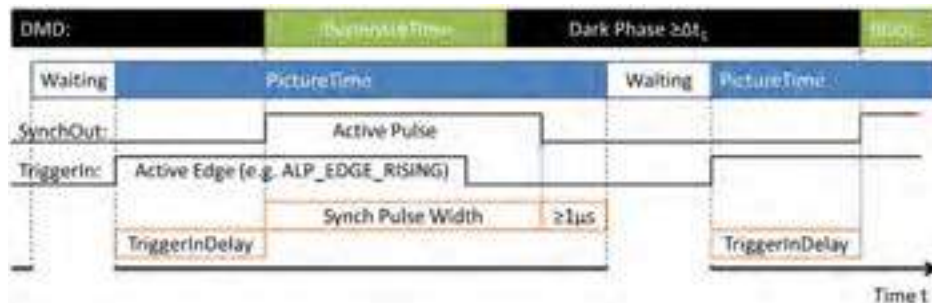
Figure 6: DMD timing in slave mode
