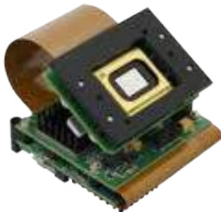
Figure 5: Digital Micromirror Device and its controller
