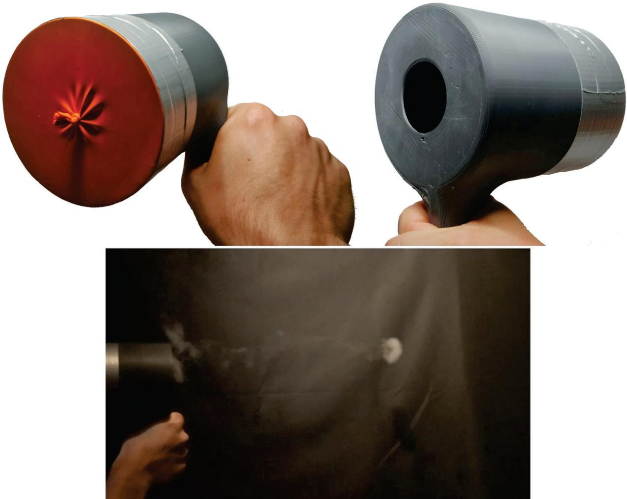
Fig. 27. Design of a simple DIY smoke vortex cannon. The barrel is 3D printed and a cut balloon is used as membrane.
