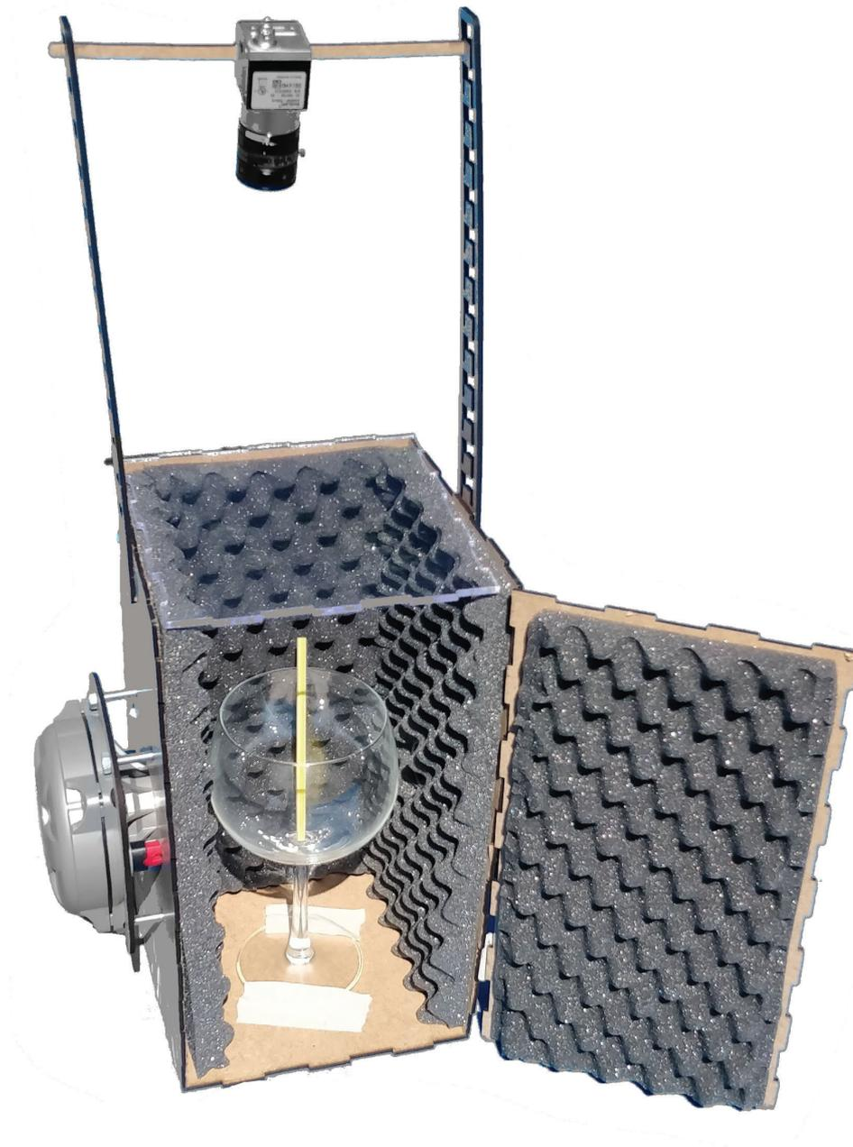
Fig. 26. Setup for the glass breaking experiment, comprising a laser cut sound-proof box, two compression speakers and a 750fps camera.
