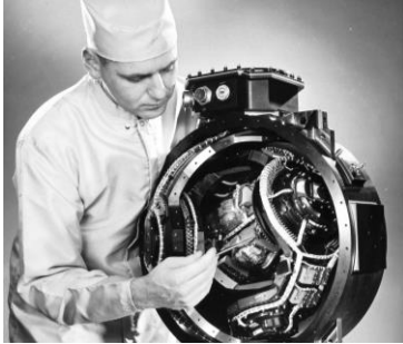
IMU on Saturn V (1960)
