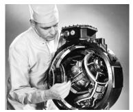
IMU on Saturn V (1960)
